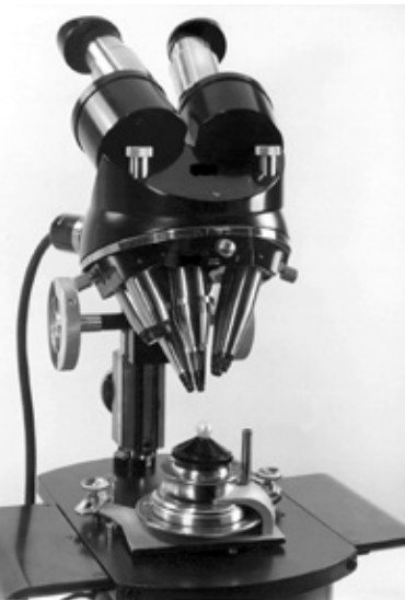
Eduard Josef Gübein also developed instruments for examining gemstones, such as this gemmoscope, a binocular microscope with dark-field illumination.
